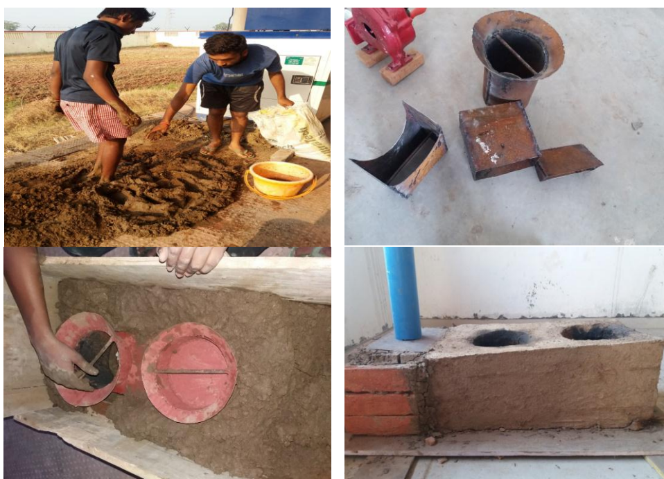
Figure1. Fabrication of two pot advance chulha
